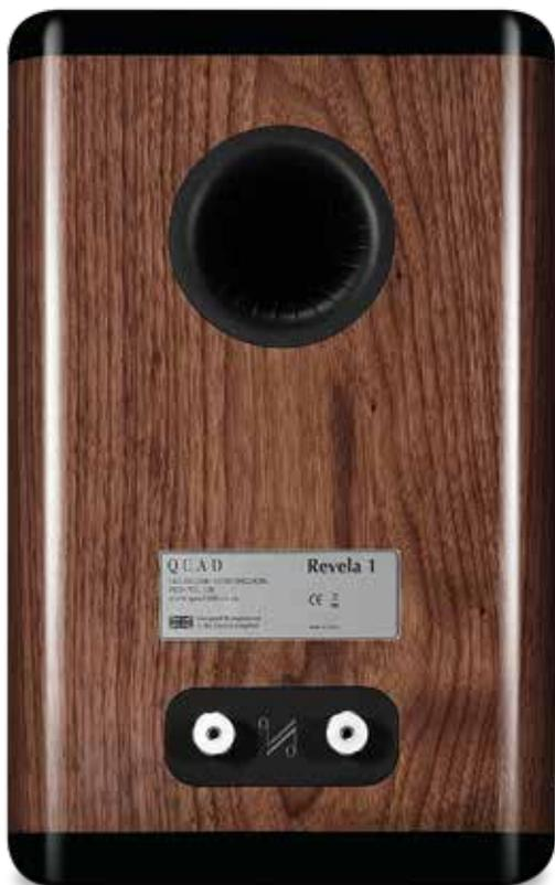
**LEFT:** The Revela 1's two-way 'phase-compensated Acoustic Butterworth' crossover does not support bi-amping or bi-wiring – hence the single 4mm cable binding posts. The large reflex port includes longitudinal splines to smooth the airflow at low bass frequencies
